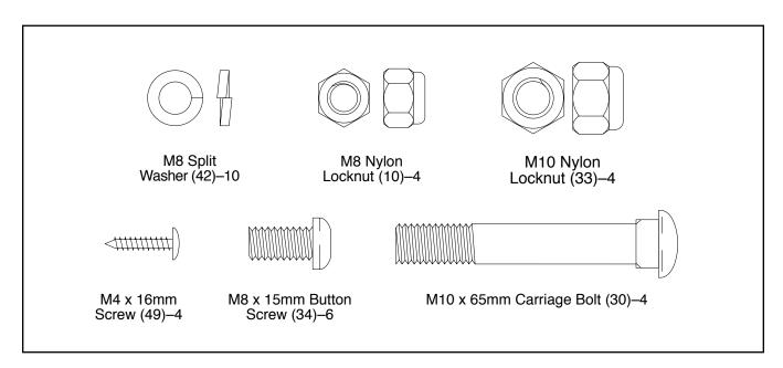
While another person lifts the front of the Frame (1) slightly, attach a Stabilizer (2) with two M10 x 65mm Carriage Bolts (30) and two M10 Nylon Locknuts (33).
